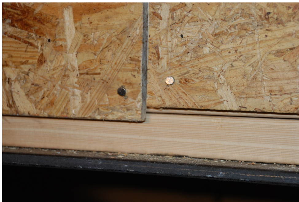
Figure 4.126: Displacement of panels after Fatigue 1 test of Specimen C-3C
