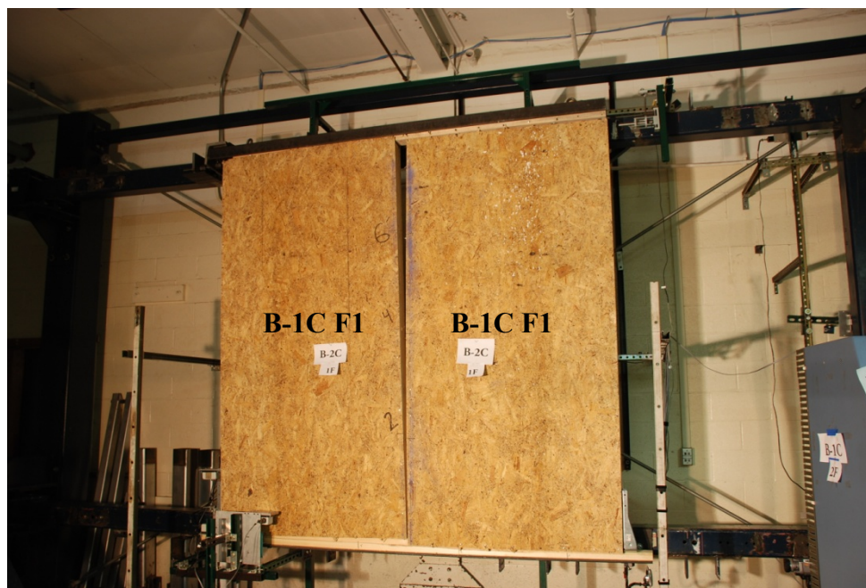
Figure 4.91: Displacement of panels in relation to each other after Fatigue 1 of Specimen B-1C
