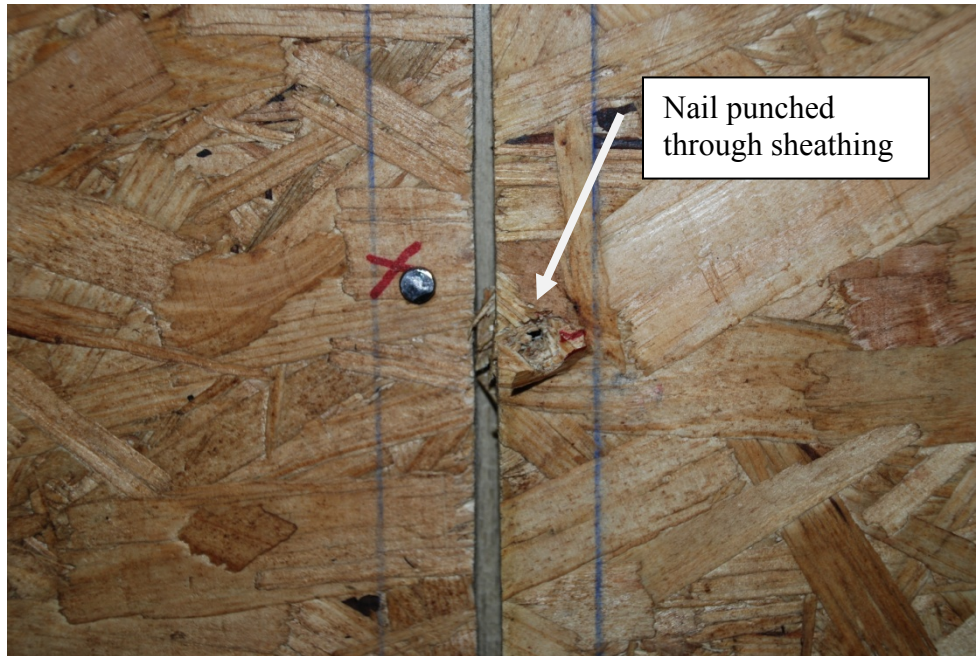
Figure 4.120: Punch through of nail along spline of Specimen C-2C after Fatigue 2 test
