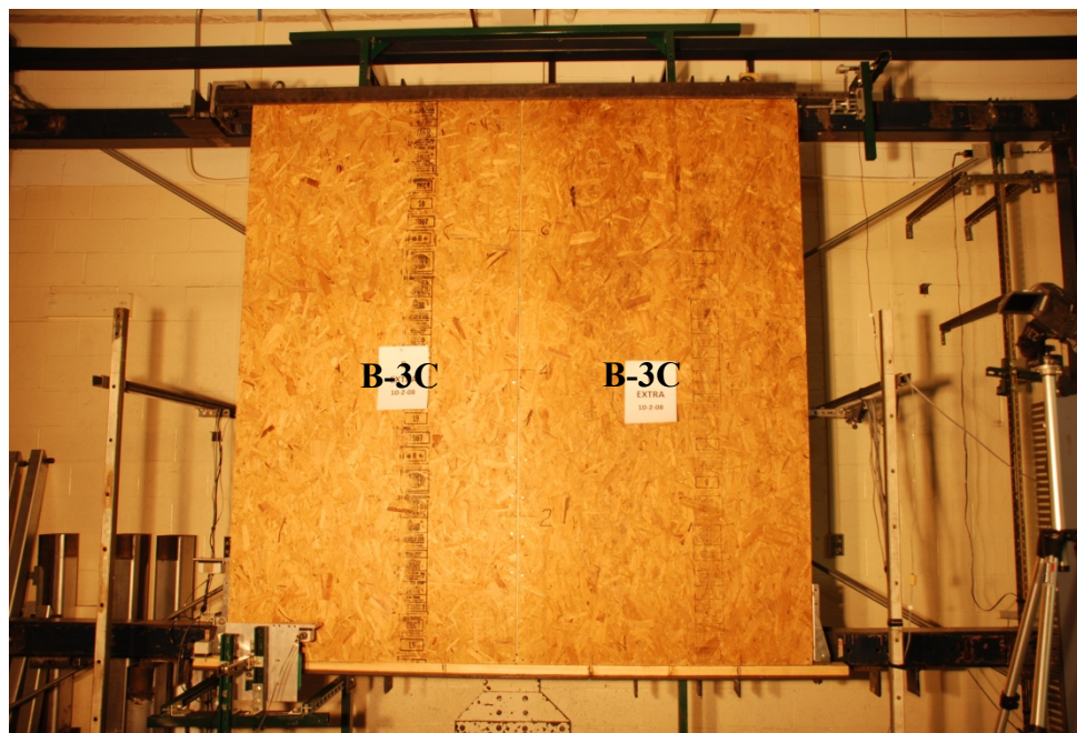
Figure 4.105: Specimen B-3C on test facility prior to cyclic loading
