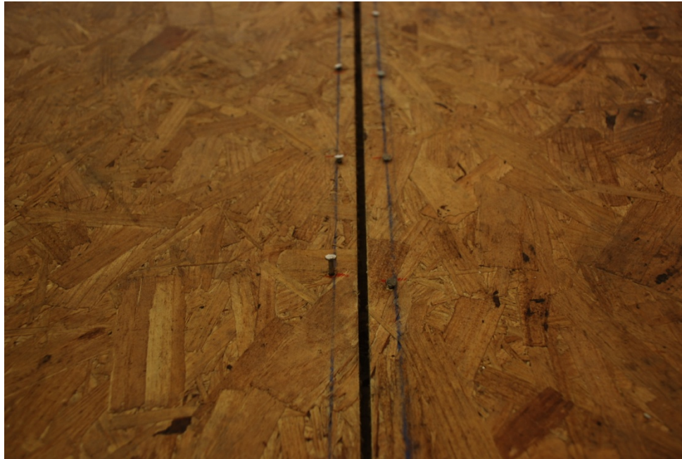
Figure 4.69: Nail pull-out along spline of Specimen A1Bearing-3C after Fatigue 1
