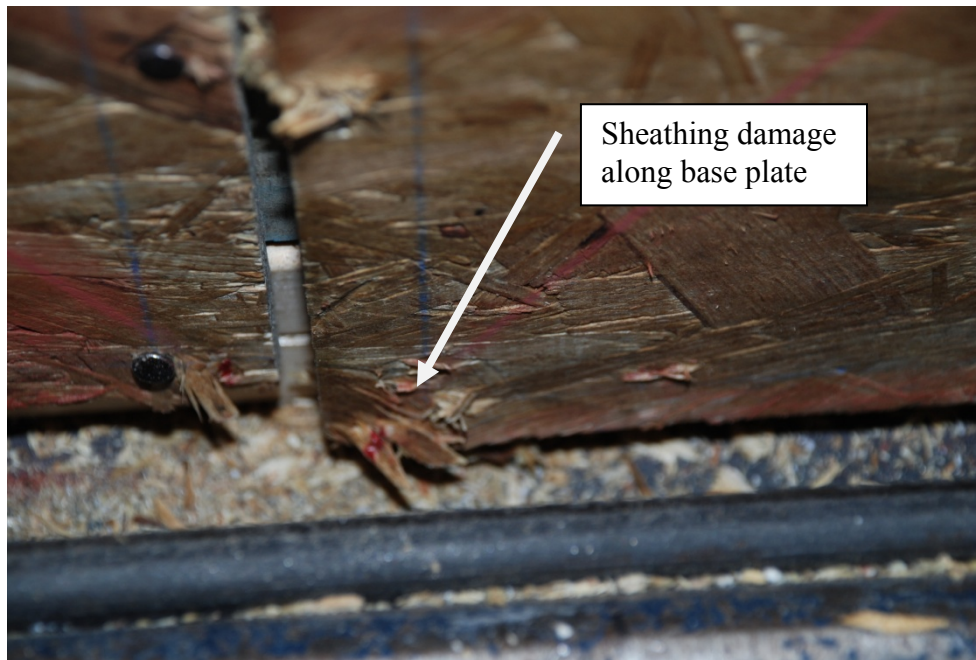
Figure 4.122: Damage to sheathing along base plate of Specimen C-2C after Fatigue 2 test
