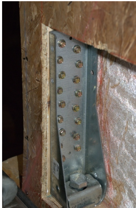
Figure 4.75: Internal USP PHD6 hold-down fit into 13.5 in.x15.5 in. cut-out in SIP panel of Specimen A1Internal-4C
