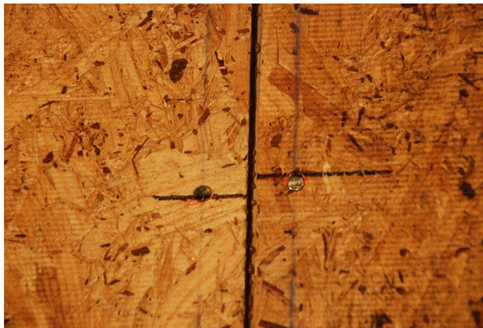
Figure 4.101: Horizontal and vertical deflection of Panel 1 and Panel 2 along spline of Specimen B-2C after the Fatigue 2 test
