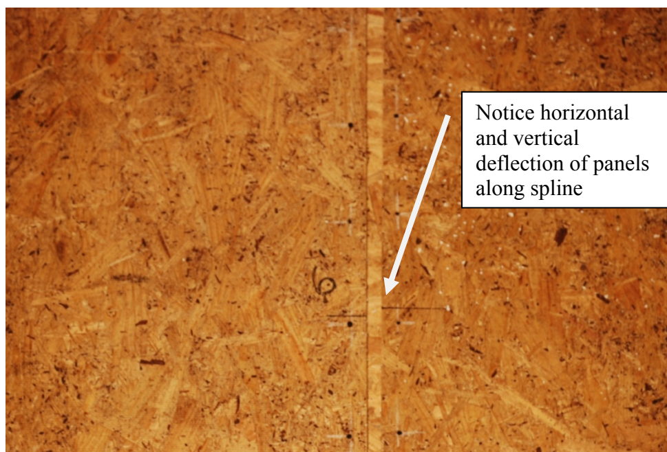
Figure 4.25: Deflection of SIP panels six feet high on Specimen A4-1C after cyclic loading
