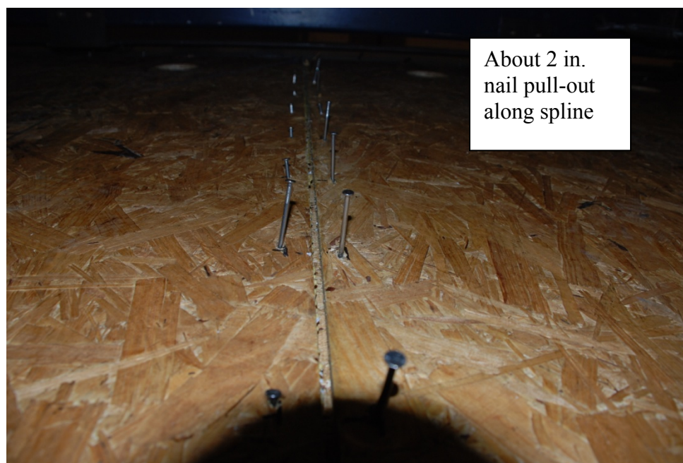
Figure 4.49: Nail pull-out along spline of Specimen A1-1C after Fatigue 3
