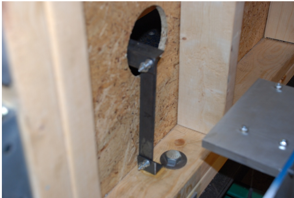
Figure 3.19: Z shaped metal piece attached to base plate and LVDT in order to measure deflection
