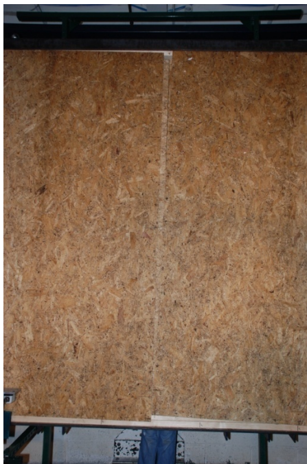
Figure 4.18: Deflection of SIP panels after the monotonic loading of Specimen A4-1M
