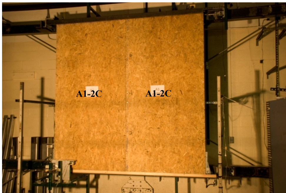
Figure 4.53: Specimen A1-2C prior to cyclic loading
