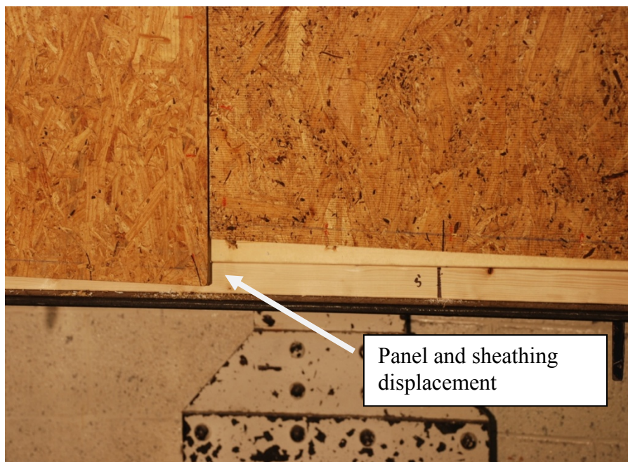
Figure 4.10: Displacement of panels along base plate and vertical sliding of SIP panels after cyclic loading of Specimen A3-2C
